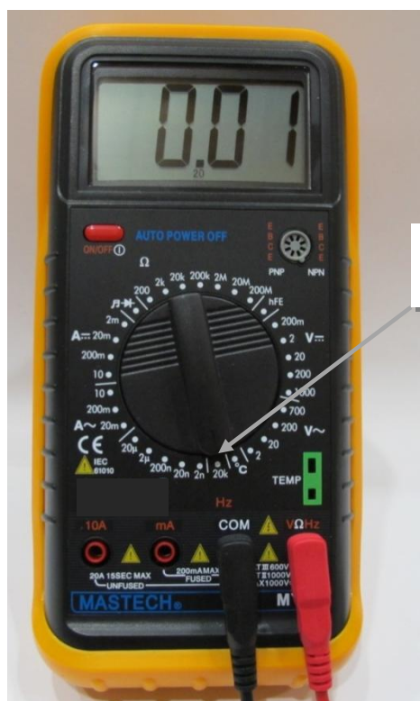
FIGURE 3 Digital multimeter for measuring frequency
